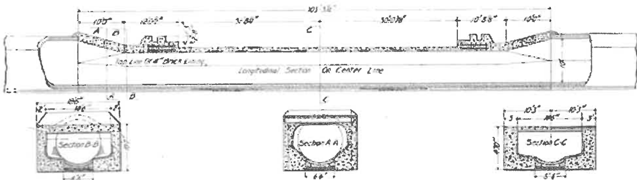
Brighton Beach Line—Reconstructed Sewer at Foster Avenue.
